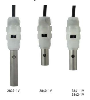
The Signet 2839-1V(D) to 2842-1V(D) Conductivity/ Resistivity Electrodes are available in four cell constants from 0.01 to 10.0 cm<sup>-1</sup>, and are suitable for a wide variety of applications from high purity water quality monitoring to weak acids and bases. 316 SS electrode surface finishes are controlled in a precision bead blasting operation to ensure measurement accuracy and repeatability.
